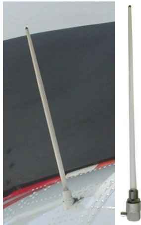
Chelton 21-41 antenna installed on a Eurocopter aircraft
