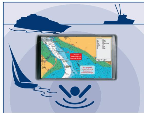
**MOB incident results in activation of AIS MOB device, which transmit a localised locating signal on maritime VHF frequencies to a range of 4 miles (appx).**
